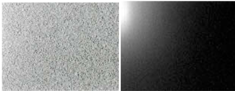
Examples of dark frames. (Left) A standard dark frame that you might see from your system; (right) a ten-minute dark frame showing amplifier glow, commonly seen in older CCD cameras.
